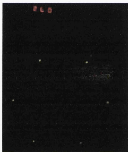
Figure 5.3: Sharp (1 X 1) LEED pattern of the UHV cleaned 4H-SiC sample, taken at 45eV.
