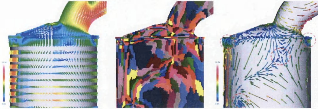
Figure 6.21: A screen shot of the visual result comparison between the direct flow visualization (left) and the feature-based visualization (right). (left) The cluttered direct flow visualization can't do a good job of extracting important flow features. (middle) Vector field clusters are generated and coloured in different colours. (right) Based on the generated clusters, shaded streamlets with arrow head are applied to reveal some flow features such as vortices and saddle points which are highlighted by red circles.
