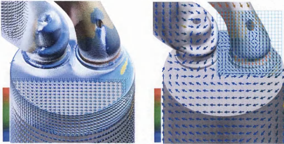
Figure 3.9: The comparison of brute-force hedgehog visualization (left) and our multi-resolution glyph-based visualization which is powered by Gaussian filter (right) applied in order to depict the flow at a surface of an intake port mesh composed of unstructured, adaptive-resolution 221K polygons. Notice how the glyphs are cluttered using the hedgehog approach (left). Also notice that the uneven appearance resulting from the underlying mesh that have nothing to do with the actual flow. Glyphs are colour-coded according to velocity magnitude.
