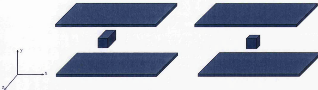
Figure 5.2. (a) 2.5 D representation of a square shaped cylinder with infinite length is placed between parallel walls. (b) in a corresponding 3D representation, the cylinder length is small and contained within the control volume e.g. a cube as shown.
