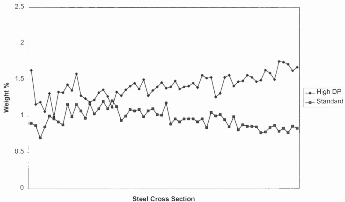
Figure 7.18: Oxygen levels for a cross section of steel C utilising both standard and high dew point annealing conditions from EDS analysis.
