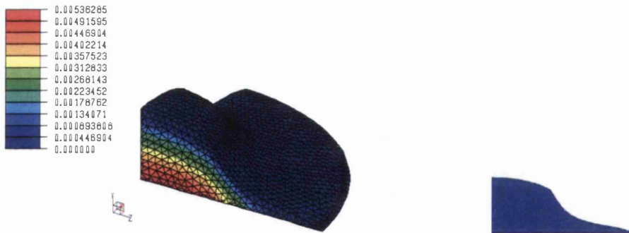
Figure 5.21c Pressure contour at t = 0.3 , (H/R) = 0.4042
