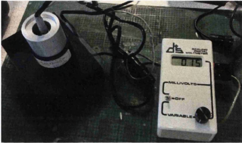
Figure 3.8: Emissometer measuring the emissivity of 7.5 \Omega/\square FTO glass
