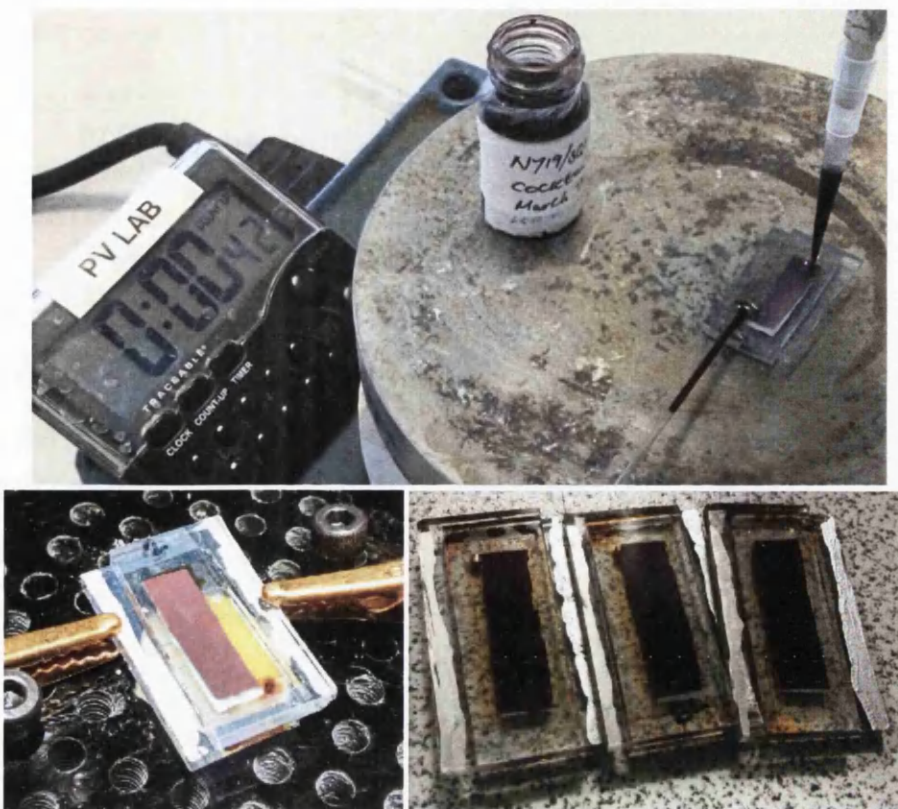
Figure 8.6: Dyeing of a shell in progress (above) and finished devices (below)
