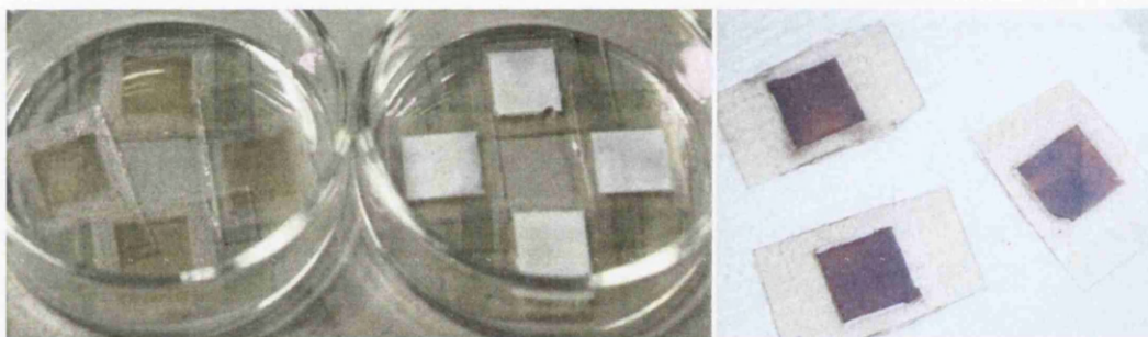
Figure 2.13: Working electrodes with Surlyn prior to dyeing (left) and after (right)
