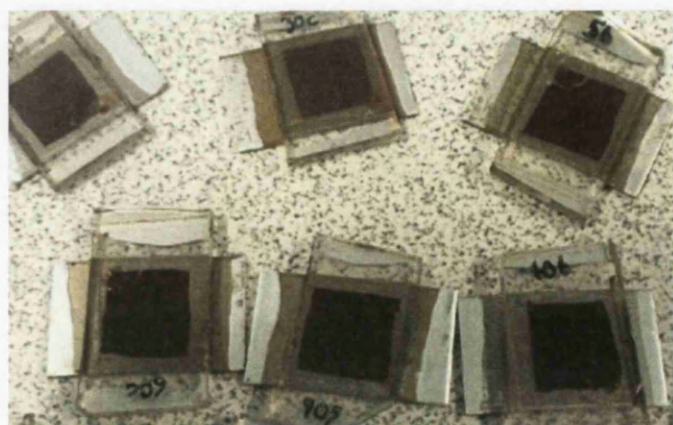
Figure 2.12: Metal counter electrodes DSCs with the working electrode drilled
