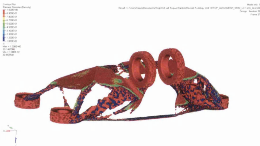
Figure 5-25: Topology Optimisation with Loadcase 1 only applied
