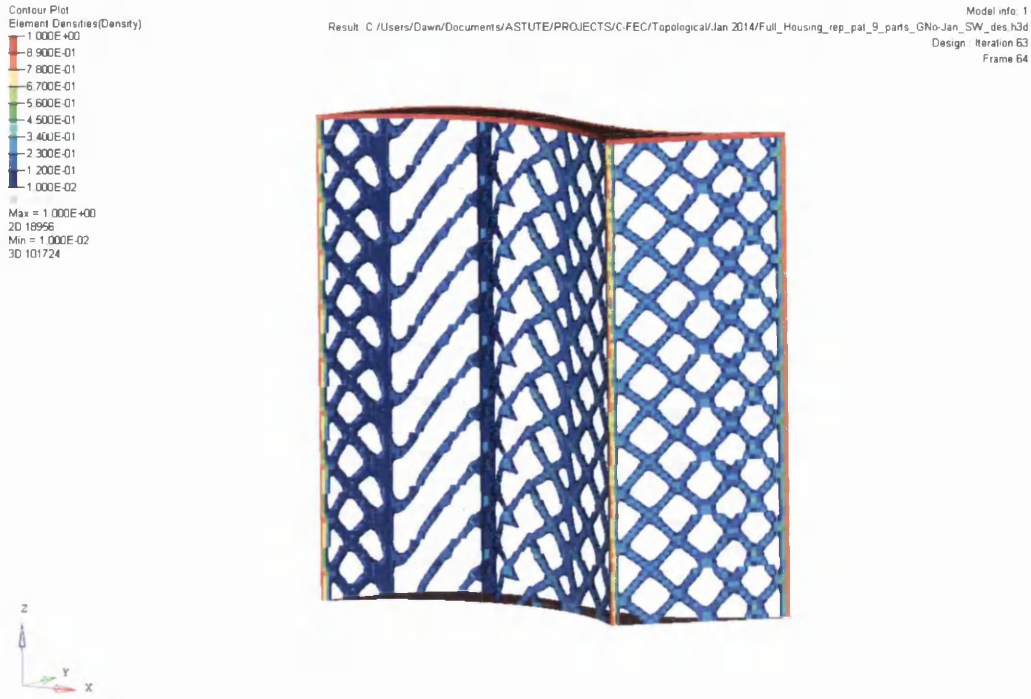
Figure 3-13: Result of Topology Optimisation of Complete Housing with pattern repeat in nine sections
