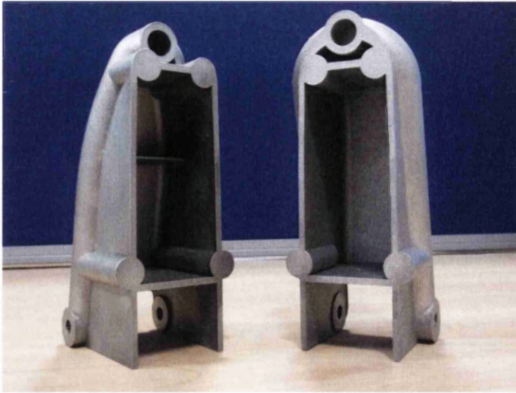
Figure 7-23: ALM built Casing parts
