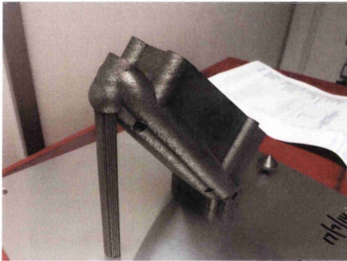
Figure 7-24: ALM Part B affixed to base with Support material still attached
