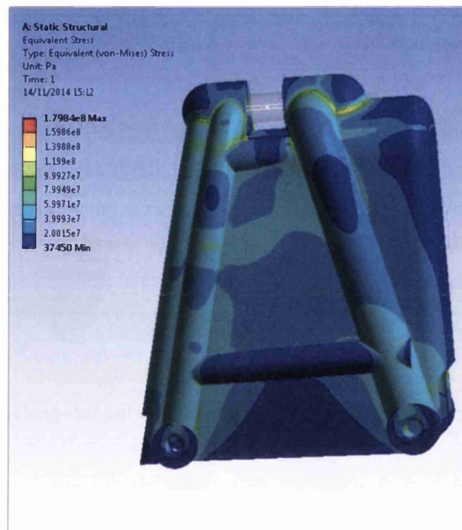
Figure 7-16: Stress contours from Linear Static Analysis of Optimised Casing under 45kN load
