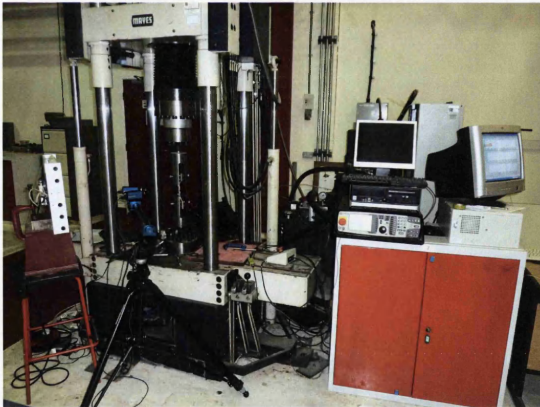
Figure 6.15. Mayes fatigue testing equipment
