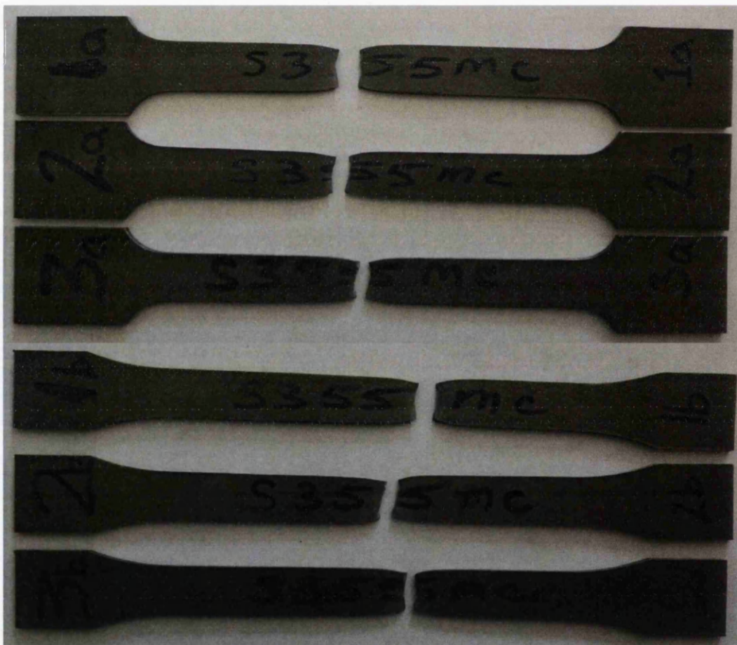
Figure 3.6. Failed S355MC tensile specimens
