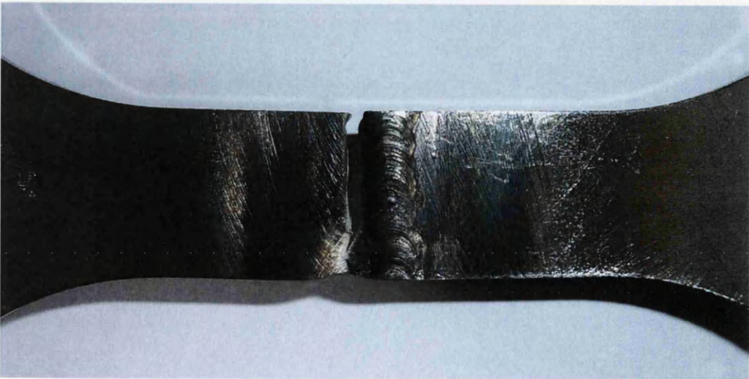
Figure 6.27. Over-performing TIG weld Failure
