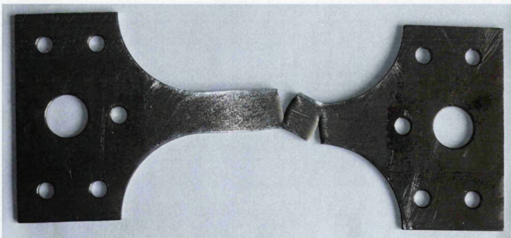
Figure 3.9. Two fatigue cracks that grew concurrently
