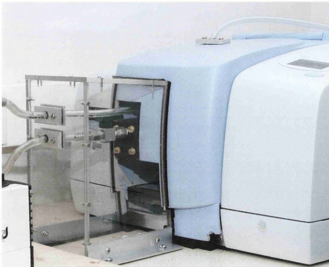
Figure 1.47 – Close-up of Gas Cell within the FTIR Sampling Compartment
