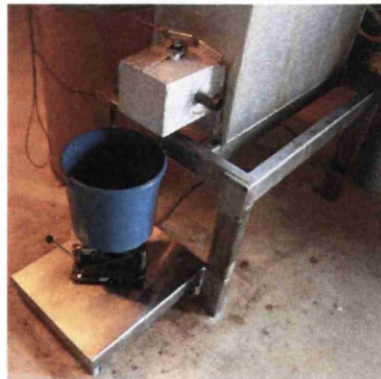
(f) Drain valve (sampling point)
