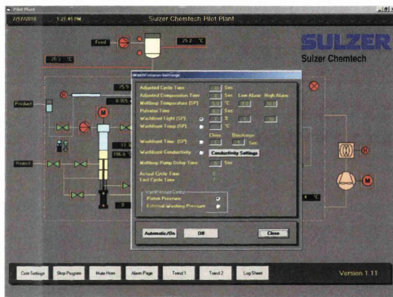
Fig. 6.14: Screen shot of the pilot plant software with a dialog window of wash column settings.
