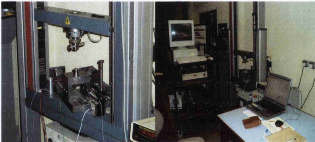
Figure 3.2 Actual Apparatus of Extended Sliding Plate
