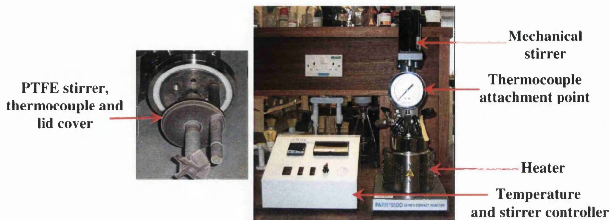
Figure 2.5. PTFE liner and automated stirring autoclave
