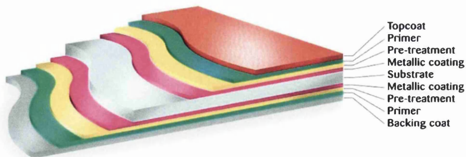
Figure 5.1. A typical composition of organic coated steel, image courtesy of Corus (© Corus) 121 .
