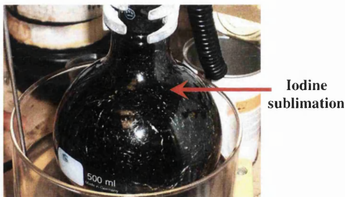
Figure 2.4. Iodine sublimation during direct iodination of phthalimide
