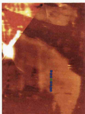
Figure 6.8: Example of a shear-force topography image (revealed top left corner) overlaid with a high resolution contact mode AFM image and markers indicating a series of TERS measurement positions. The measurement positions are defined based on the shear-force image. Features are matched between the shear-force and AFM images to ensure accurate alignment is achieved.
