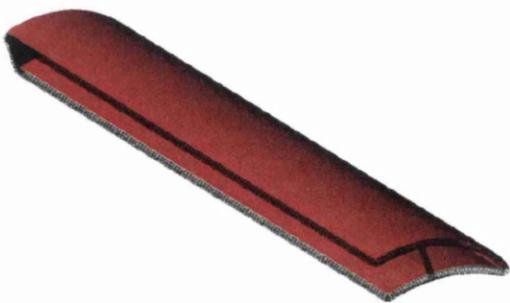
Figure 7.17: A typical FE model. Due to symmetry only 1/4 of the blade is modeled.
