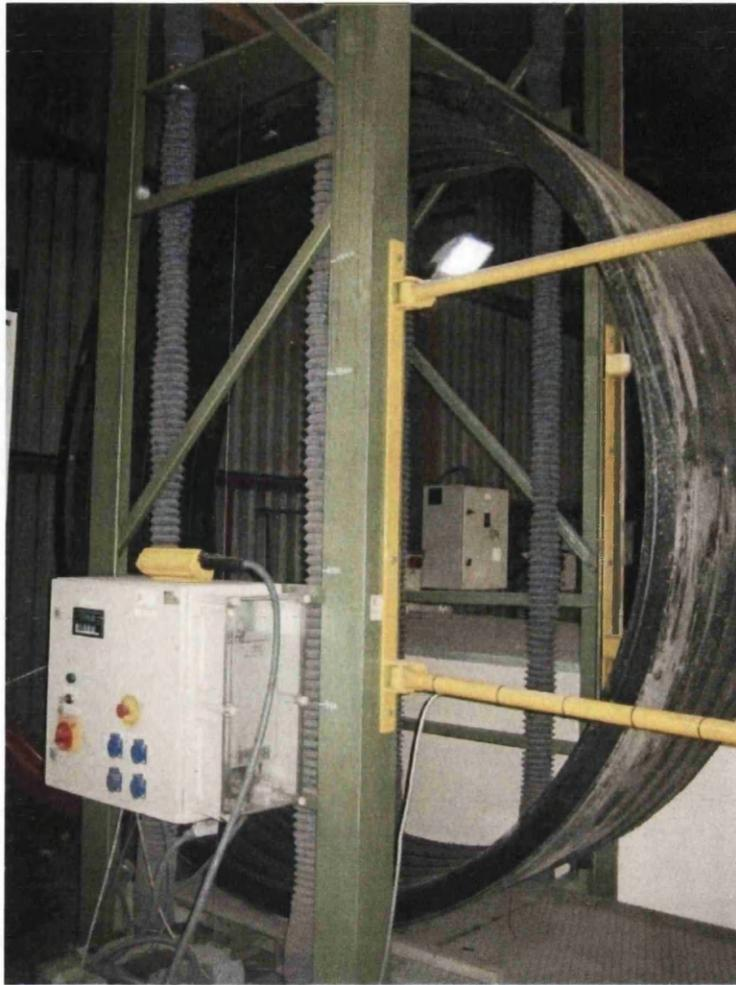
Figure 5.13: Pipe placed in the ringstiffness machine. The pipe is compressed in between two horizontal plates up to a vertical deflection of 3% of the internal diameter.
