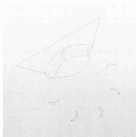
Figure 7.2: While the rotor is in motion the blades pass through a tunnel. To avoid obstruction the displacements of the blades' tips have to be constrained.
