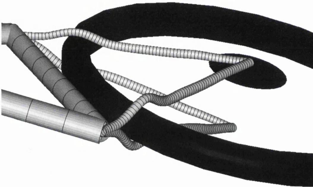
Figure 6.22: Penalized boundaries for tyre and disc brake obstruction constraint. The small circle at the rear drop out represents the disc brake and the surface in between the stays represents the tyre.
