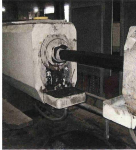
Figure 5.5: The extruded profile is cooled down until it reaches the desired temperature for winding it onto the mandrel.
