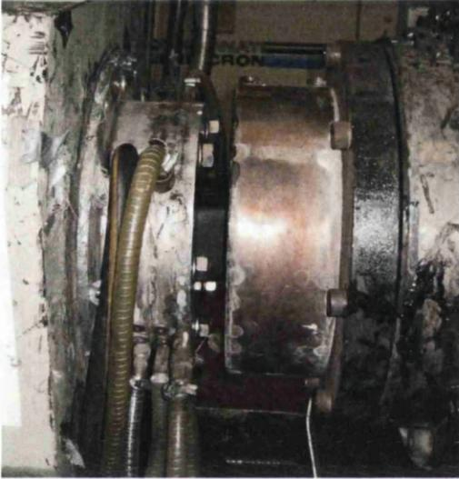
Figure 5.4: The HDPE granules are melted and using vacuum pressure formed into the desired profile.
