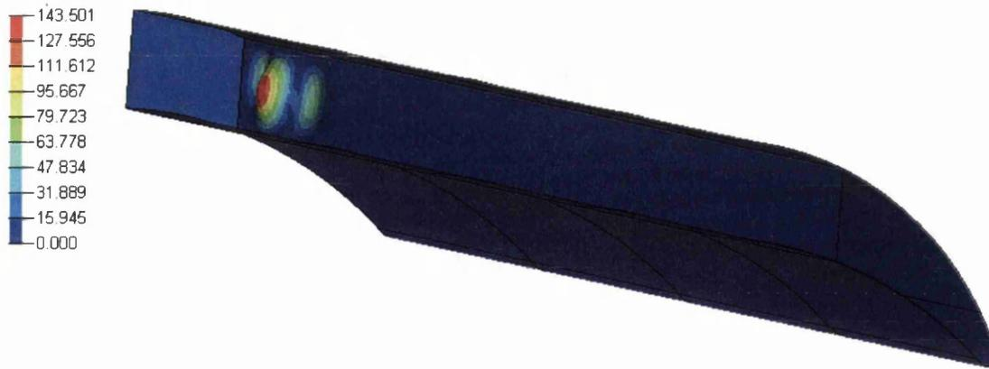
Figure 7.30: Contour plot of the first buckling mode for load step 1. The corresponding EV is 9.83 and the minimum allowable EV is 1.5. The buckling occurs in the web near the support. In case of buckling the maximum displacement is 143.5mm for this mode.
