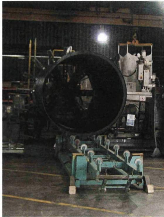
Figure 5.7: The pipe grows on the rotating mandrel and is gradually moves along its axis.
