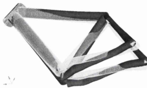
Figure 6.4: Deformed shape for the Out-of-saddle rigidity test.
