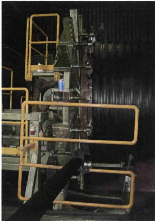
Figure 5.6: The extruded HDPE profile is wound around the mandrel and continuously welded to the adjacent one.
