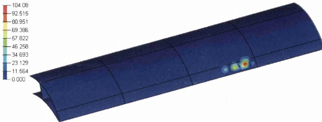
Figure 7.31: Contour plot of the first buckling mode for load step 2. The corresponding EV is 5.64 and the minimum allowable EV is 1.5. The buckling occurs on the top surface on the side of the blade. In case of buckling the maximum displacement is 104.1mm for this mode.
