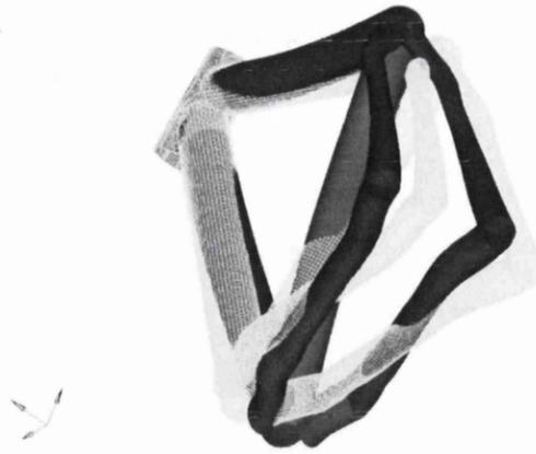
Figure 6.8: Deformed shape for the Out-of-saddle test.
