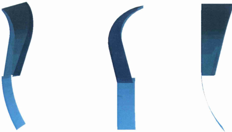
Figure 163: Option 2 revised curved chute insert design
