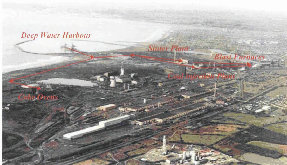
Figure 1: Aerial view of Port Talbot integrated steel works showing raw material conveyor belt distribution links
