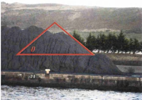
Figure 137: Coal \theta = 41 degrees and DEM simulation \theta = 43 degrees
