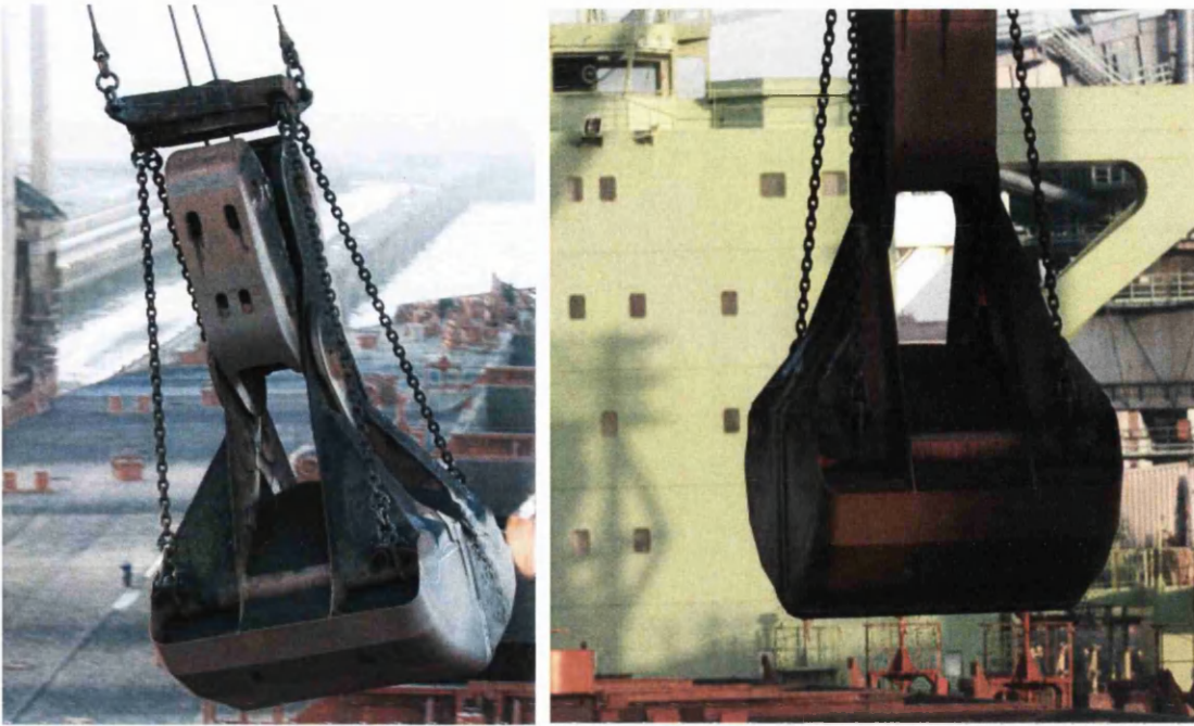
Figure 139: Grab moves along a gantry boom carrying material over to the unloader hopper
