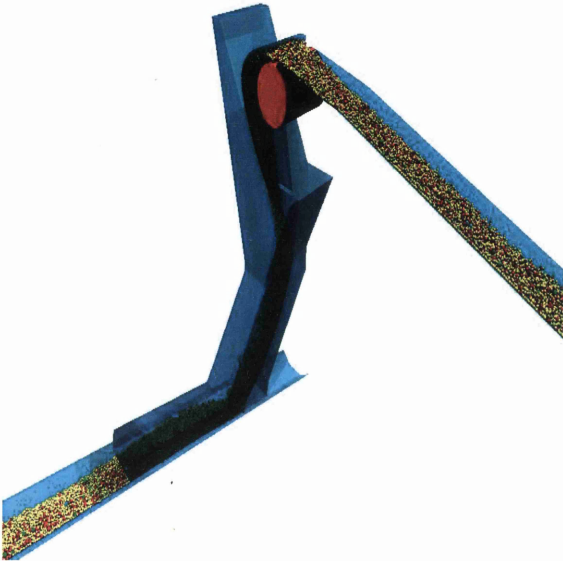
Figure 157: 633-634 Head Chute with curved inserts
