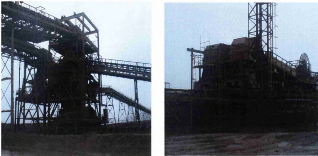
Figure 2: Conveyor belt transfer stations used to redirect raw material flow
