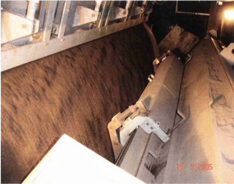
Figure 10: Shows the roll feeder with supply gates releasing raw mix
