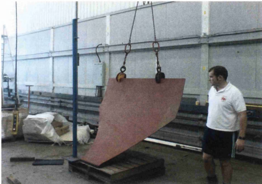
Figure 69: The curved chute suspended from the gantry crane.
