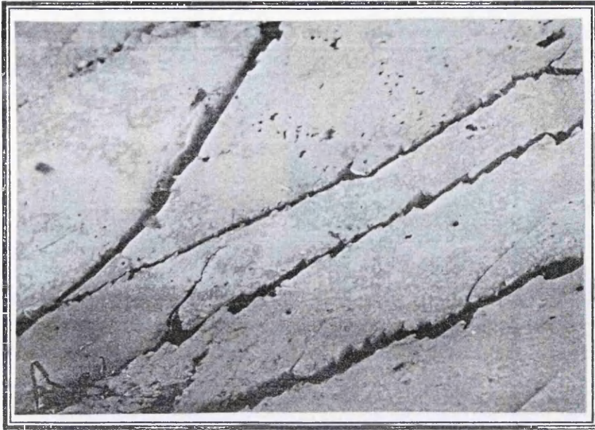
Figure 5.48: Cracks can be seen near the fracture surface. Sample [\pm 45]_4 , R=-1 , sea water, 28 MPa, N_f=755 , 25X.
