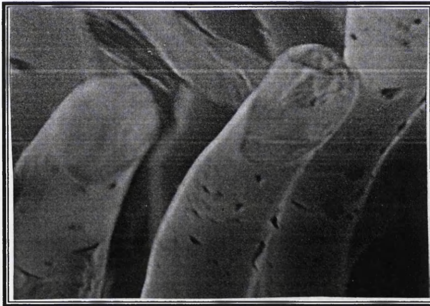
Figure 5.51: The image shows brittle fibres fracture. Sample [\pm 45]_4 , R=-1 , air, 60 MPa, N_f=195 , 1000X.
