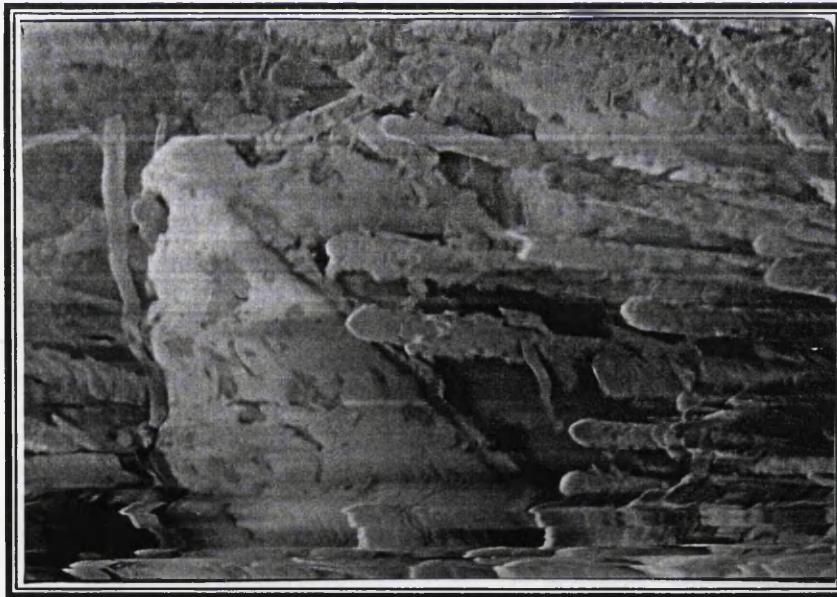
Figure 5.80 : SEM: Modulus degradation fracture surface showing fibre pull out and some matrix still attached to fibre. Sample [\pm 45]_4 , R=-1 , 40 MPa, N_f= 16218 , 200X.
