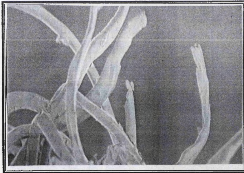
Figure 5.45: Bundle of \pm 45^\circ fibre pull out. Sample [\pm 45]_4 , R=0.1 , distilled water, 21 MPa, N_f = 131825 , 170X.
