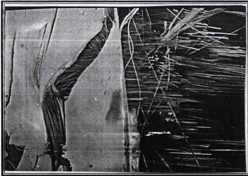
Figure 5.37: The same type of cracks observed near the fracture surface. Sample [90^{\circ}/0^{\circ}]_{2S} , R=0.1 , air, 180 MPa, N_f=3573 , 15X.
