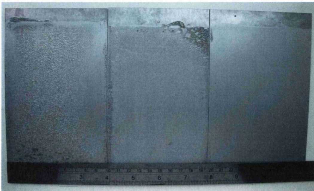
Figure 5.9 – Corresponding Substrate Panel Topside (from Figure 5.8), Cured with Same NIR Settings with Silver Top Coat
