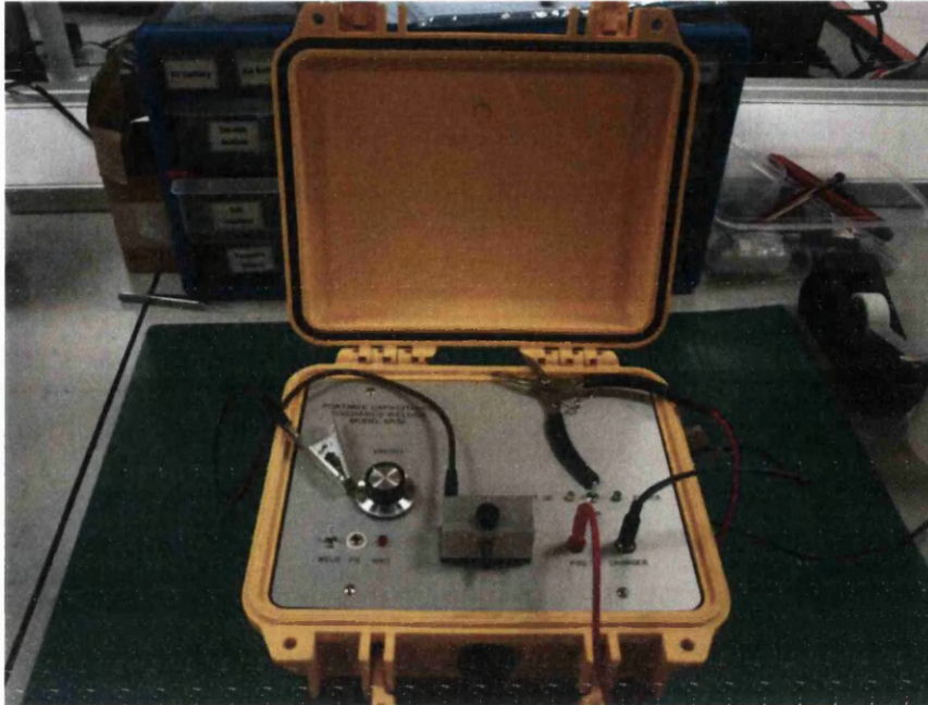
Figure 2.6 - SR 50 Capacitance Discharge Welder used to Spot Weld Thermocouples
