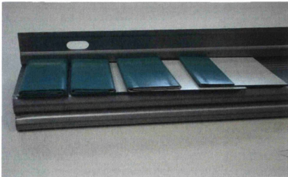
Figure 1.30 – T Bend Test - reproduced from [28]
