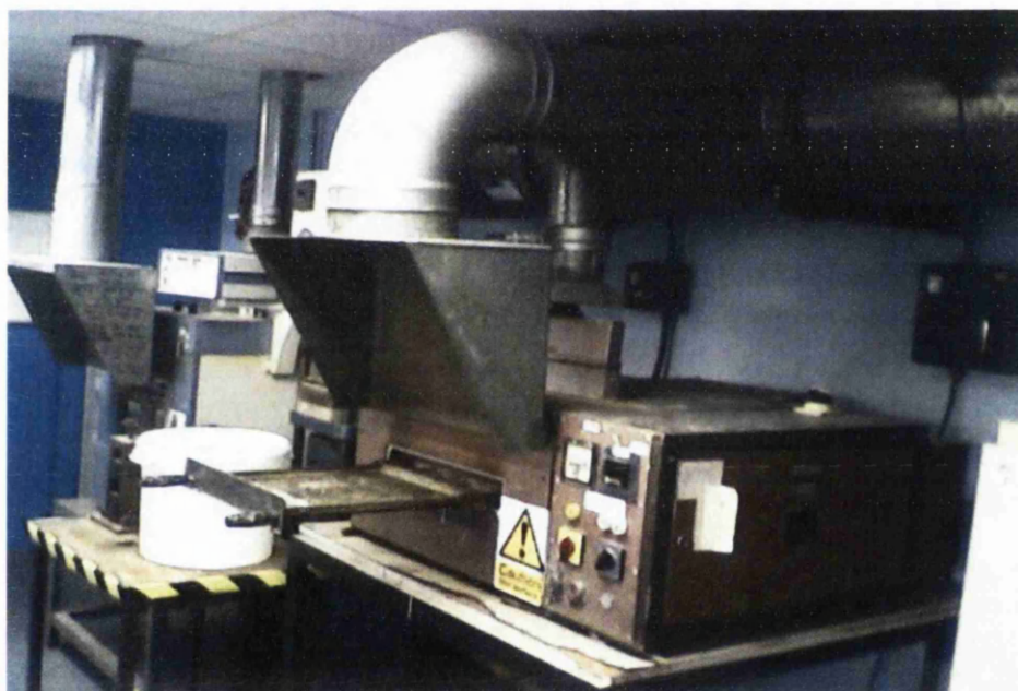
Figure 2.8 – Mathis Oven for Convection Cure of Polyester Coatings
