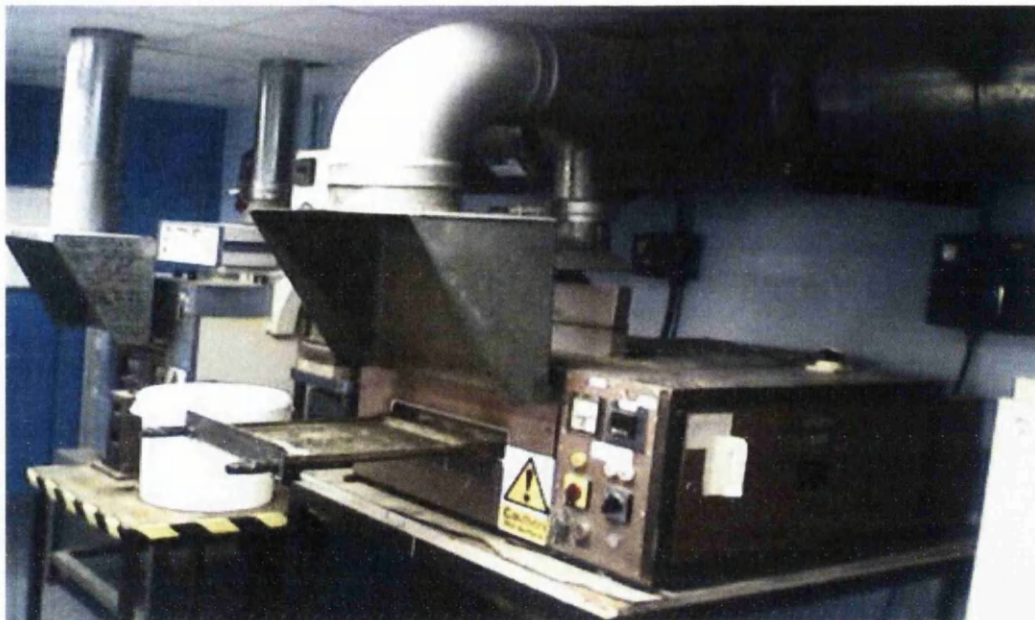
Figure 4.12 – Mathis D70 Convection Oven with Timed Automated Entry and Exit
