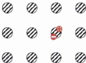
Figure 1.6 The electron-hole pair in a Frenkel exciton.
