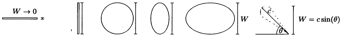
Figure 4.13: With horizontal oscillating inflow, structures with these cross-section shapes all have the same added mass per unit length equation of \rho\pi(W/2)^2 dl where W is the facing width.
