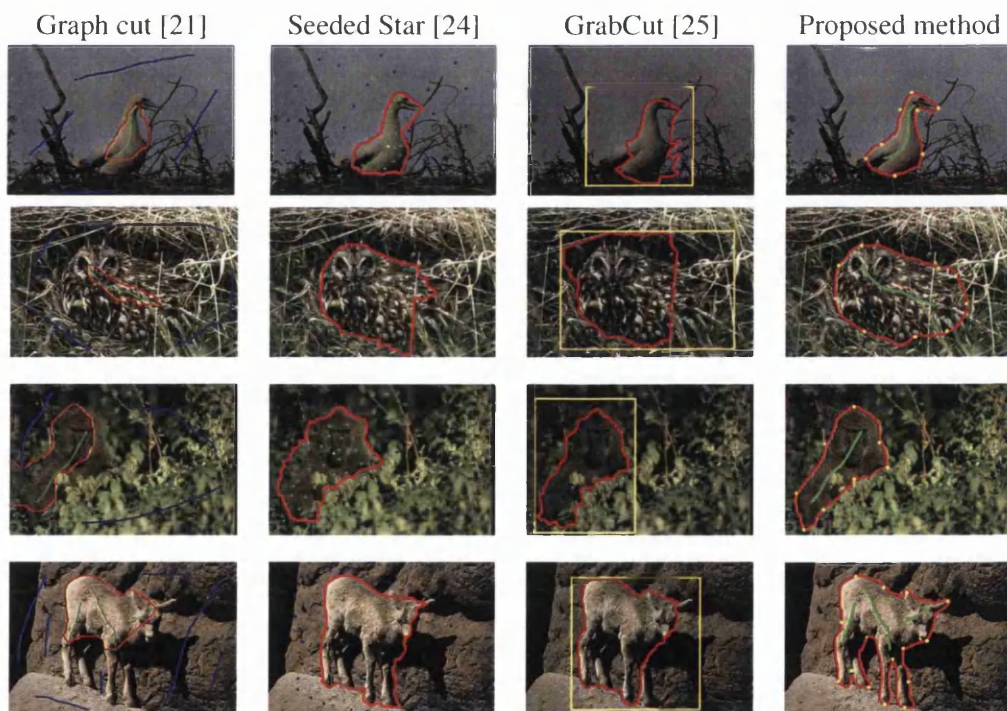
Figure 3.20: Segmenting animals from complex scenes. From left: Graph cut [21], Seeded Star Graph Cut [24], GrabCut [25], and proposed method. Red curve shows the segmentation result, blue for the background strokes, green for foreground strokes, and yellow for star point and the initial window of the Grabcut.
