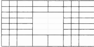
Figure 43 – The (i,j,k) structure of a mesh with hanging nodes
