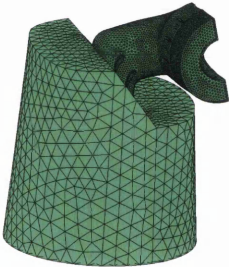
Figure 117 – The Unstructured Mesh around the Engine
