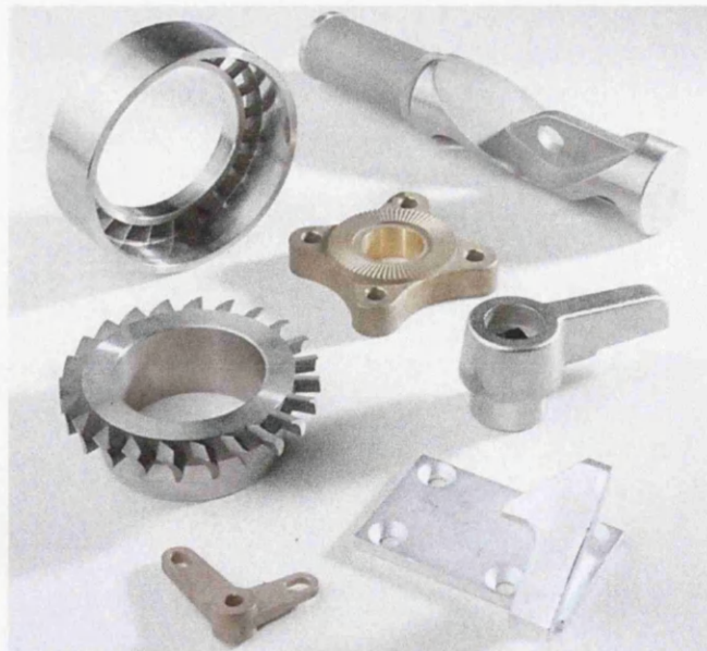
Figure 2.5.3: Examples of the complex geometry components that can be produced by the MIM process [52].
