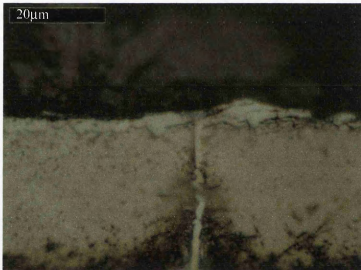
Figure 5.5.3: A high magnification optical micrograph showing evidence of primary \alpha growth remote of the Ti-6-4 substrate material.
