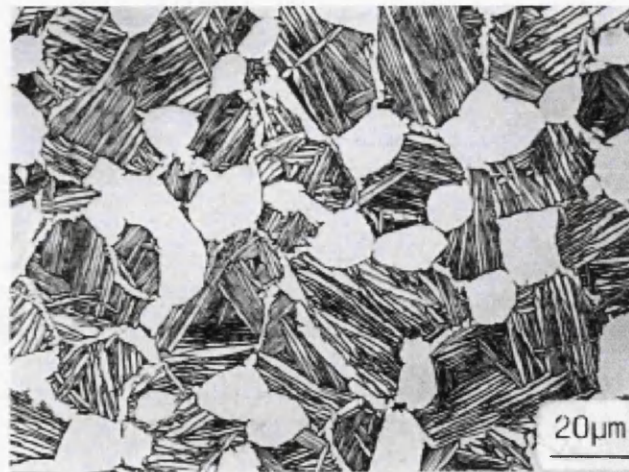
Figure 2.2.2: Typical bi-modal structure observed in Ti-6242 [12].
