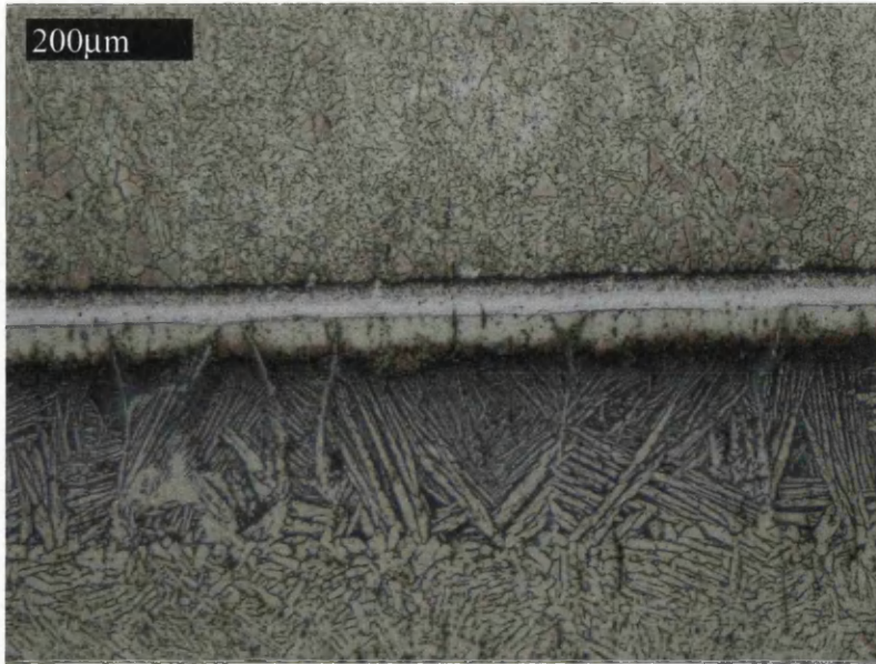
Figure 5.5.1: An overview of the interfacial microstructure of Test 33b (IN718 to Ti-6-4 including Cu braze).
