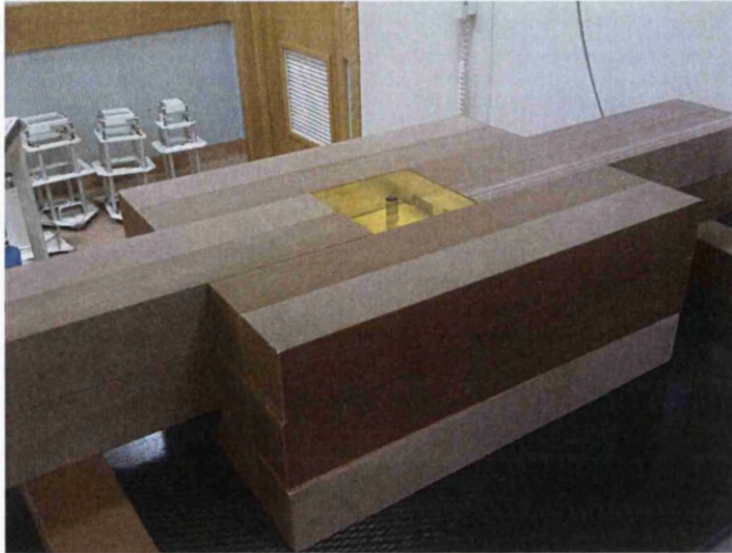
Figure 5.5: Experimental set up of the irradiation of the diamond detector with the 6 MV photon beam. The diamond detector sits in the middle of a PMMA cubic phantom of 8 cm side and is surrounded by the WT1 multiblock phantom.
