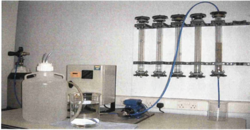
Picture 1. Activated Unsaturated Sand Filter
