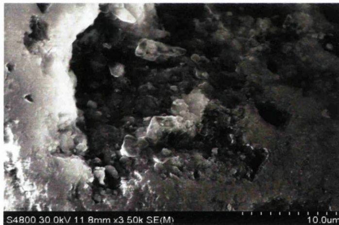
Figure 4.17 SEM micrographs for mixed metals bearing coated sand at 3,500x magnification ( d_{sand} = 0.710\text{mm} , q_{Mn}/q_{sand} = 0.0709 \text{ mg Mn/g sand} , C_{in} = 20 \text{ mg/L} )
