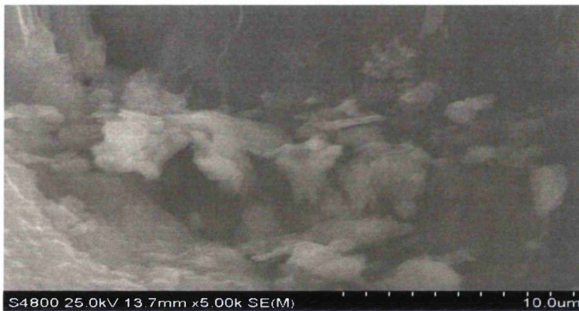
Figure 4.7 SEM micrographs for copper bearing coated sand at 5,000x magnification ( d_{sand} = 0.710\text{mm} , q_{Mn}/q_{sand} = 0.0709 \text{ mg Mn/g sand} , C_{in} = 20 \text{ mg/L} )
