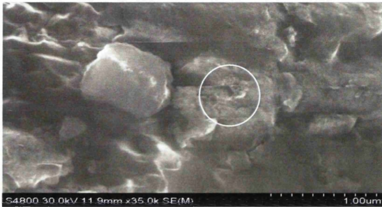
Figure 4.8 SEM micrographs for manganese bearing coated sand at 35,000x magnification ( d_{sand} = 0.710\text{mm} , q_{Mn}/q_{sand} = 0.0709 \text{ mg Mn/g sand} , C_{Mn-in} = 20 \text{ mg/L} )
