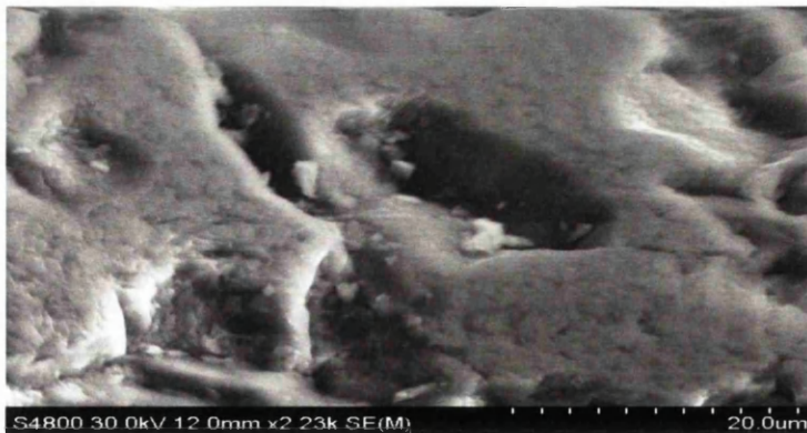
Figure 4.19 SEM micrographs for waste water bearing coated sand at 2,230x magnification ( d_{sand} = 0.710\text{mm} , q_{Mn}/q_{sand} = 0.0709 mg Mn/g sand, C_{Cu-in} = 11.78 mg/L, C_{Mn-in} = 0.061 mg/L, C_{Zn-in} = 0.6135 mg/L, C_{Ni-in} = 0.81 mg/L)
