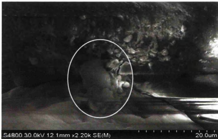
Figure 4.15 SEM micrographs for nickel bearing coated sand at 2,200x magnification and 30.0kV ( d_{sand} = 0.710\text{mm} , q_{Mn}/q_{sand} = 0.0709 \text{ mg Mn/g sand} , C_{Ni-in} = 20 \text{ mg/L} )
