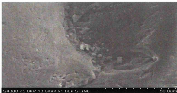
Figure 4.5 SEM micrographs for copper bearing coated sand at 1,000x magnification ( d_{sand} = 0.710\text{mm} , q_{Mn}/q_{sand} = 0.0709 \text{ mg Mn/g sand} , C_{Cu-in} = 20 \text{ mg/L} )
