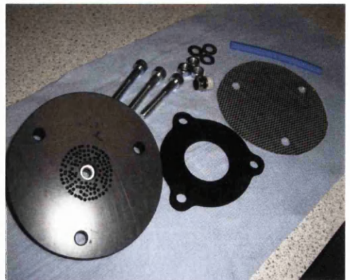
Picture 5. Bottom perforated plate together with its accessories i.e. perforated screen (mesh), rubber plate, bolt and a plastic hose
