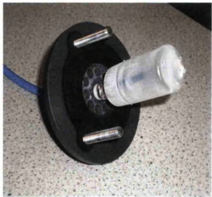
Picture 4. Top perforated plate along with its spray tube
