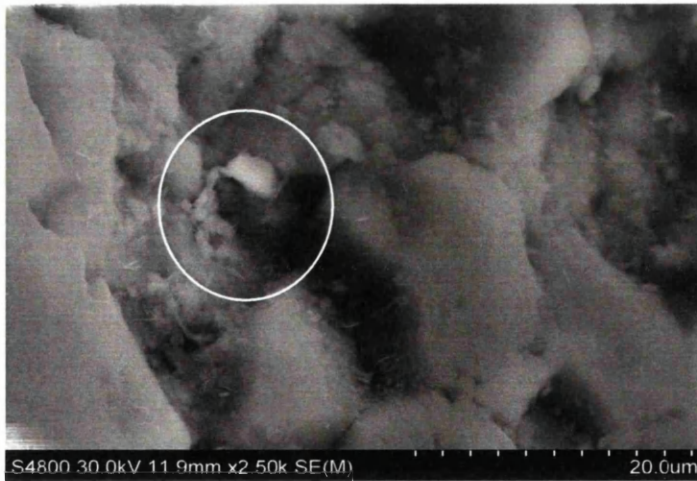
Figure 4.11 SEM micrographs for zinc bearing coated sand at 2,500x magnification ( d_{sand} = 0.710\text{mm} , q_{Mn}/q_{sand} = 0.0709 \text{ mg Mn/g sand} , C_{Zn-in} = 20 \text{ mg/L} )
