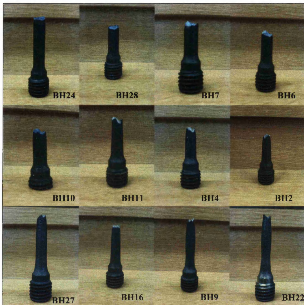
Figure 25: Photos taken from the 12 creep exposed Esshete 1250 specimens.
