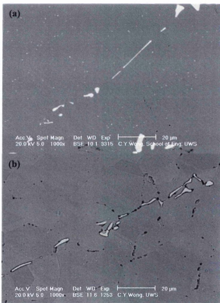
Figure 36: SEM micrographs used for image analysis and manual point counting of volume fraction. (a) un-etched condition, (b) etched with oxalic acid solution.
