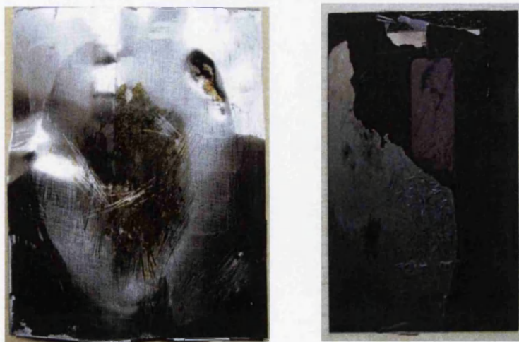
FIGURE 5.5 (b): One year old ECCS based DSC substrate coated with 90% TiN/PI coating shows no significant signs of corrosion (Right) Uncoated ECCS substrate exposed to DSC electrolyte (Left).
