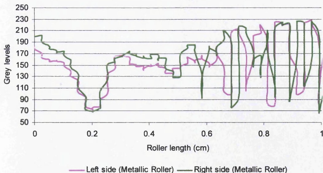
Figure 6-15 Ribbing increases locally at the sides of the roller which determine a lateral flow and gap generation according to the ink film thickness (graph at 0.2cm rollers length). The graph suggests that ribbing width is formed equally between the two sides of the same roller. This indicates that the nip gap is the same along the rollers nip length. The top image illustrates the captured ribbing image. The bottom graph visualise the grey levels of the green and red areas of the top picture in order to compare the density of the lateral areas of the rollers. The green area is rotated in order to match the two grey levels lines into the same graph.
