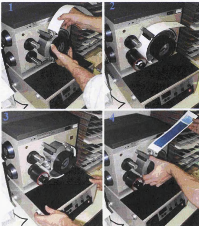
Figure 3-20 The substrate strip is mounted on the printing sector (1) and is set in printing position (2). Ink is transferred by impression with the inked printed disc (3). The printed sample is removed for drying (4) and further analysis.
