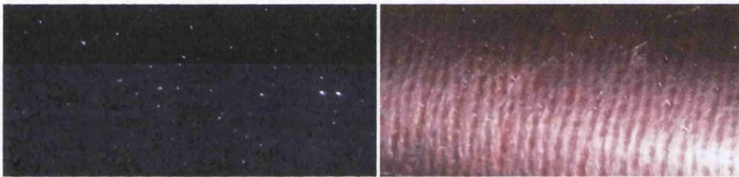
Figure 9-10 The trapped air comes on the surface of the elastic (left) and the metallic (right) roller after distribution stopped.
