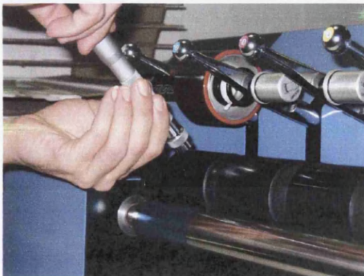
Figure 3-18 Ink volume is applied by a micrometer pipette on the IGT high speed unit
