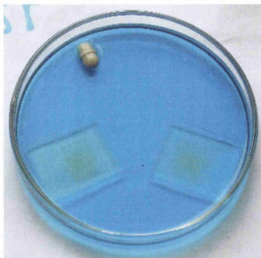
Figure 2-6 Working electrodes in dye solution (SQU 1); the dye concentration was about 3 \times 10^{-4} M
