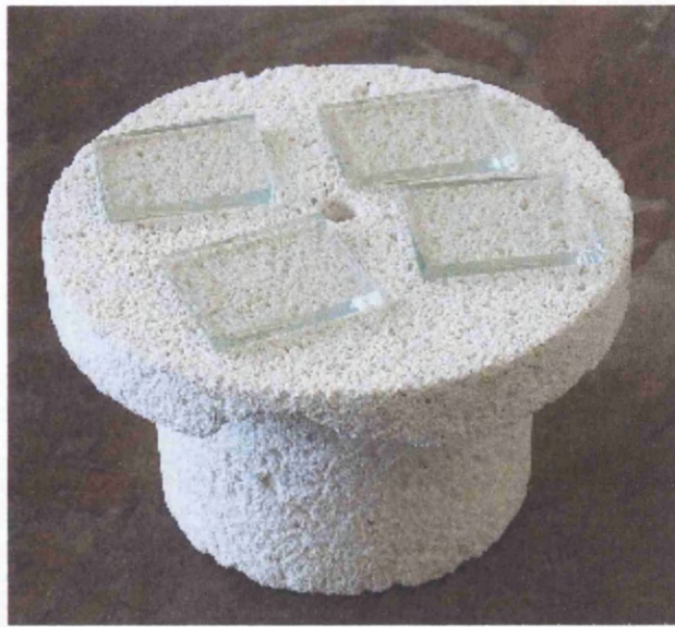
Figure 2-8 the counter electrodes before firing after the tape was removed
