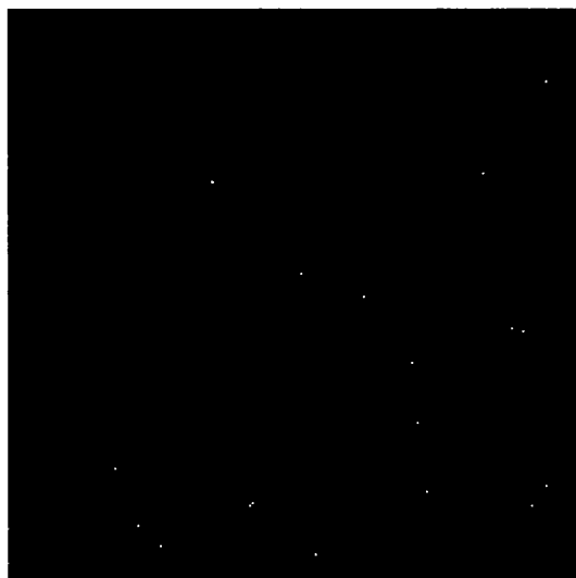
Figure 6.14. SIMS derived mass image detecting Fe^+ on a FFC attacked Zn-Al-Mg (Magizinc) alloy after the organic layer and all corrosion products had been removed from the FFC tails. Not able to show FFC tracks.
