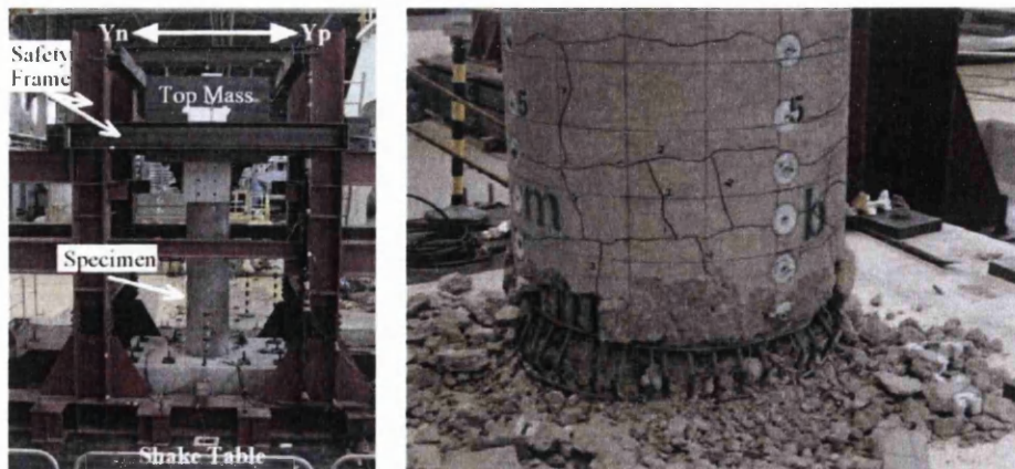
Figure 2.11 Set-up of RC specimen and the resulting damage [49]
