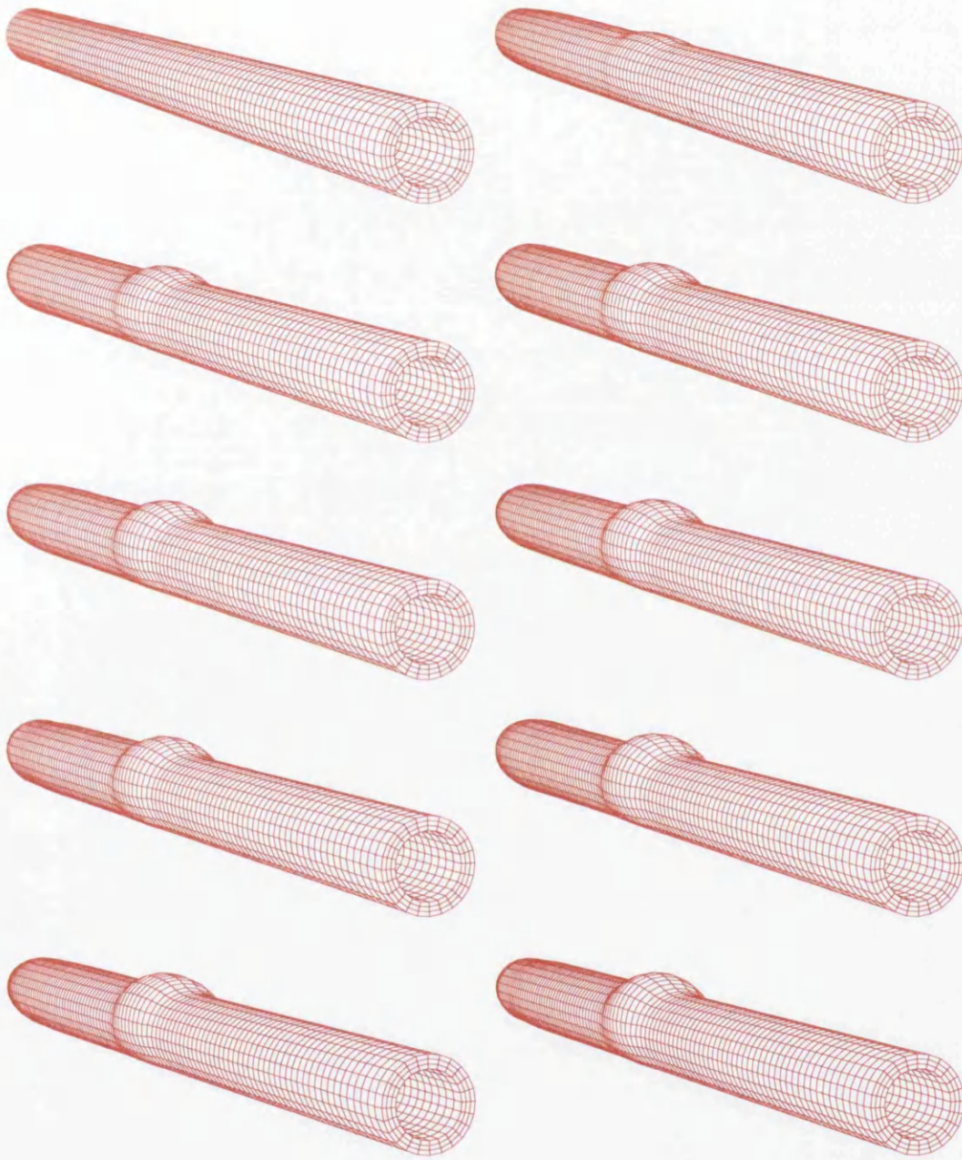
Figure 9.14: Solid mesh behavior of the weakened pipe with inner solid boundary translation fixed.
