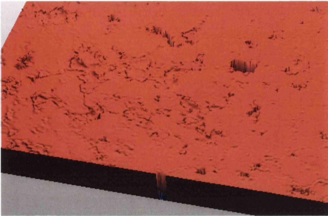
Figure 5.17 An enlargement of the section of the compact in Figure 5.15 c). 150 kN Normal load, 0.5% Lubricant
