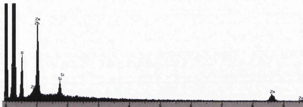
Figure 4.23 Spectral analysis of admixed lubricant (Carbon is off the scale)
