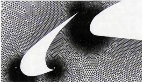
(a) Zoom of nose region of the main largest element and front element of the aerofoil
