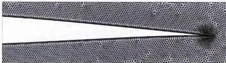
(c) Close up of tail region of SD aerofoil, displaying ten boundary layer
