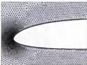
(b) Close up of nose region of SD aerofoil, displaying ten boundary layers
