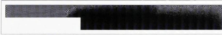
Figure 6.30: Section of mesh used to simulate flow over a backward facing step. Displays the refined region around the step. The mesh contains 53,427 elements, 27,287 nodes and 1,145 boundary nodes.
