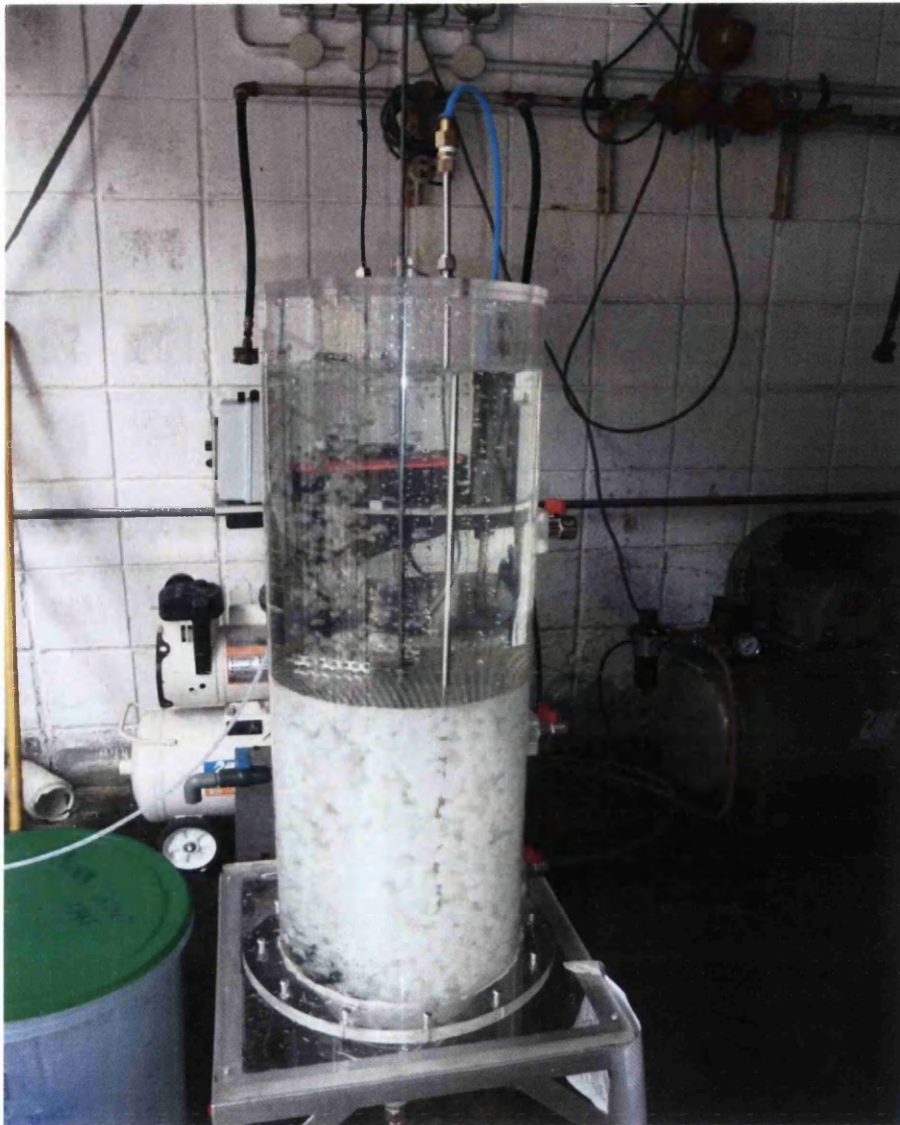
Figure 5.2: Photograph of Continuous Reactor for a Partial Fixed Bed with K2 AnoxKaldnes packing material (PFBR).
