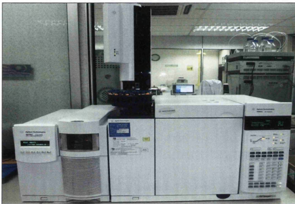
Figure 4.13: Gas chromatograph-mass spectrometer (GC-MS) model 7890A equipped with a 5975C inert MSD with a triple axis detector and a CN 93901609 autosampler (Agilent Technologies).
