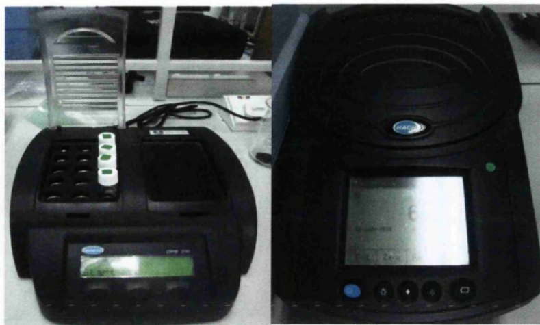
Figure 3.11: A) DRB 200 Reactor Hach. B) Spectrophotometer for COD LR Hach
