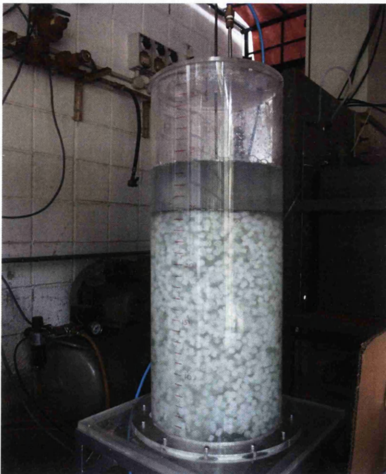
Figure 5.16: Photograph of continuous reactor for moving bed K2 AnoxKaldnes packing material (MBBR).
