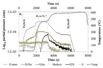
Figure 1. In situ mass spectrum of exhaust gas species after Et<sub>4</sub>Sn precursor injection as a function of time, temperature and type of carrier gas.
