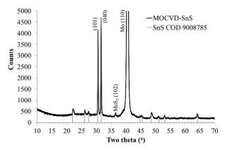
Figure 3. XRD pattern of MOCVD-grown SnS deposited at 470°C on to Mo.
