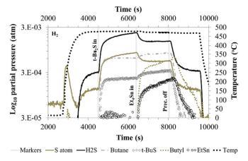
Figure 2. In situ mass spectrum of exhaust gas species after t-Bu<sub>2</sub>S injection followed by Et<sub>4</sub>Sn precursor injection as a function of time and temperature.
