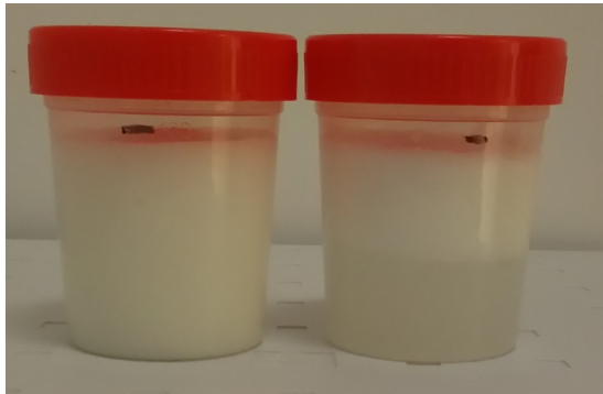
FIG. 1 Good gel phantoms have a uniform appearance (left) while failed attempts for which the microspheres have separated before solidification show distinct layers (right).
