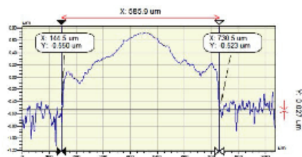
Figure 4: Cross section and width of the printed fine line measured by white light interferometry
