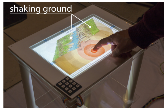
Figure 3. A user initiates a simulation with a touch gesture, and all users view the dynamic display without occluding each other, and can touch it to feel the simulation.
