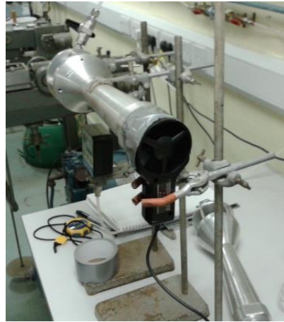
Fig. 2 The experimental set-up utilising the vane anemometer to measure the average velocity at the pre-mixer's outlet
