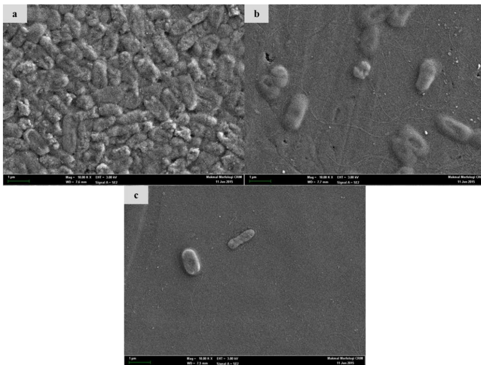
Fig. 10. FESEM images for membranes with E-coli antibacterial test: a) Pure PSF [P0] b) PSF-ZnO [Z2] c) PSF-ZnO/GO [ZG3].
