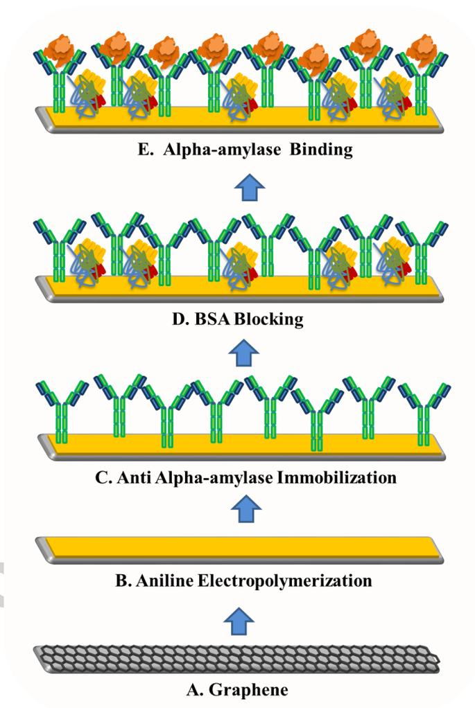
**Figure 1.** Schematic diagram for the immunosensor assembly.
