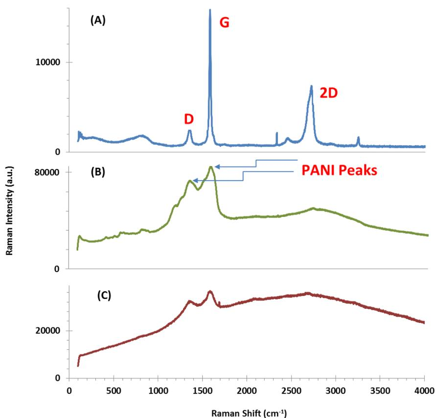
**Figure 3.** Raman spectra of (A) graphene-SPE, (B) PANI/graphene-SPE and (C) anti-alpha amylase/PANI/graphene-SPE.
