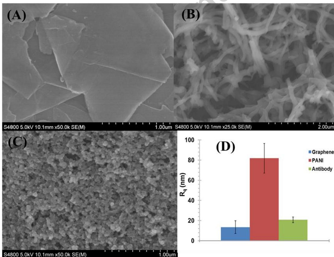
**Figure 4.** SEM images of: (A) unmodified graphene; (B) graphene modified with PANI (C); Antibody attached to the PANI layer and (D) Plot of the roughness  $R_q$  for the different samples: Graphene  $R_q = 13.5 \pm 6.36$  nm; PANI  $R_q = 81.9 \pm 14.8$  nm; Antibody  $R_q = 20.8 \pm 2.86$  nm.
