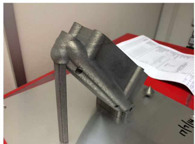
Fig. 12 ALM part a affixed to base with support material still attached
