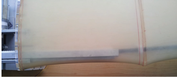
Figure 11: Poisson's contraction of the skin when fully extended.
