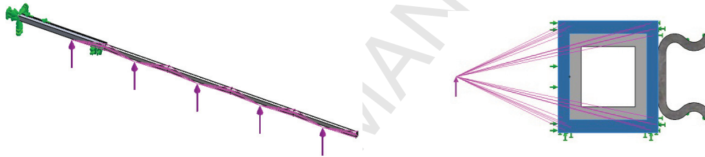
Figure 4: Nodal aerodynamic loads along the wing semispan.
