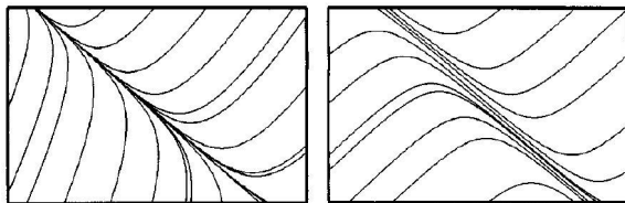
Figure 10: The vector field in the left figure contains a separation line; the field in the right figure contains an inflection line 17 .
