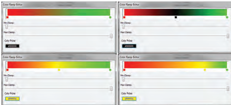
Fig. 13. Some images from an interactive session with the color map editor. The top-left image shows the initial state of the editor. The top right image shows the result when the user inserts a new sample (black) in the center of the color map. The bottom-left image shows the result after the user has updated the color of the middle sample to yellow. Finally the bottom-right image shows the effect that dragging the middle sample to right has. The color values between each sample are constructed using interpolation.
