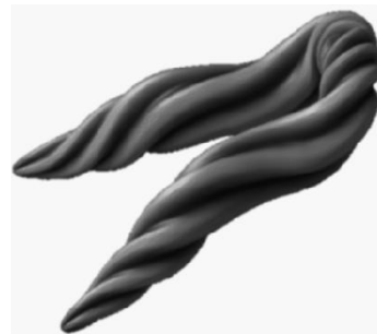
Figure 11: Reconstruction of a hairpin vortex tube, with grooves indicating velocity 2 .
