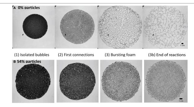
FIGURE 7 | Four phases of foam build-up for (A) a particle free experiment, and (B) a particle rich experiment containing 54 vol% particles ( $\phi \approx 1$ ). For all cases, syrup viscosity is 45–49 Pa s. Videos of these two experiments are available in Supplementary Material.
