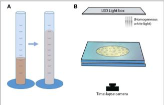
FIGURE 6 | Experimental set-up for *in situ* bubble growth using chemical reactions, in (A) graduated cylinders, and (B) parallel-plate geometry.
