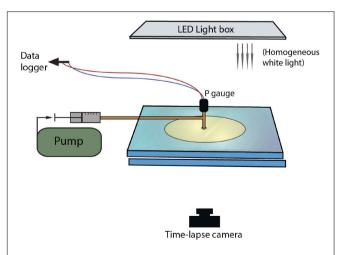
FIGURE 1 | Experimental set-up for injection of single bubbles into particle suspensions sandwiched between parallel plates.
