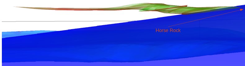
Figure 6. The eddy forming behind the Horse Rock from different angles visible (LES method).
