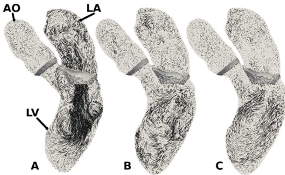
Figure 2: Slices of the left heart simulation. Velocity vectors are represented during the entering of the jet through the MV at time t = 530 ms (A) and during the late diastole phase, t = 690 ms, (B,C). (B) is an instantaneous view of the flow while (C) is the phase-averaged flow.
