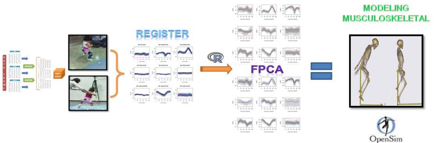
Figure 2. Methodology for inverse dynamic model using statistical modeling tool R and Opensim
