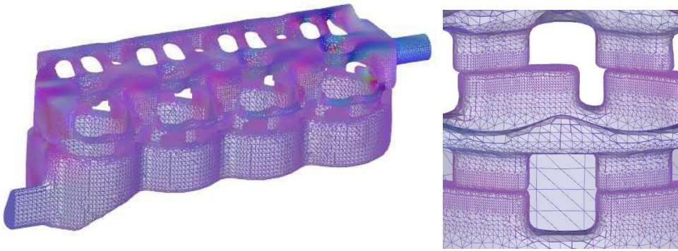
Figure 1: The unstructured adaptive resolution boundary grid of a cooling jacket from a CFD simulation. The first image is an overview of the boundary mesh, and the second is a close-up. These images illustrate how complex a typical mesh from CFD can be.
